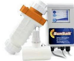
**Salt System** Salt water chlorination is a process that uses dissolved salt. The chlorine generator uses electrolysis in the presence of dissolved salt to produce hypochlorous acid and sodium hypochlorite, which are the sanitizing agents already commonly used in swimming pools. As such, a saltwater pool is not actually chlorine-free; it simply utilizes a chlorine generator instead of direct addition of chlorine.
